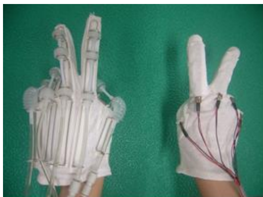
Fig.3 Master slave system of power assist hand
