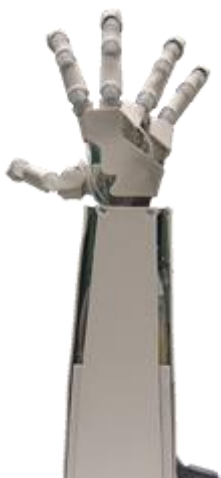
Fig.4 Robot hand with built-in pumps
