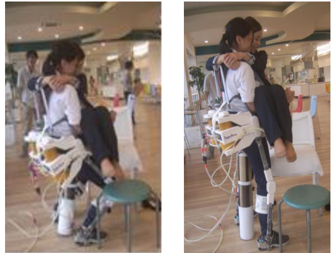
Fig.3 Care operation wearing suit with an air cylinder actuators of 100 mm \phi .
