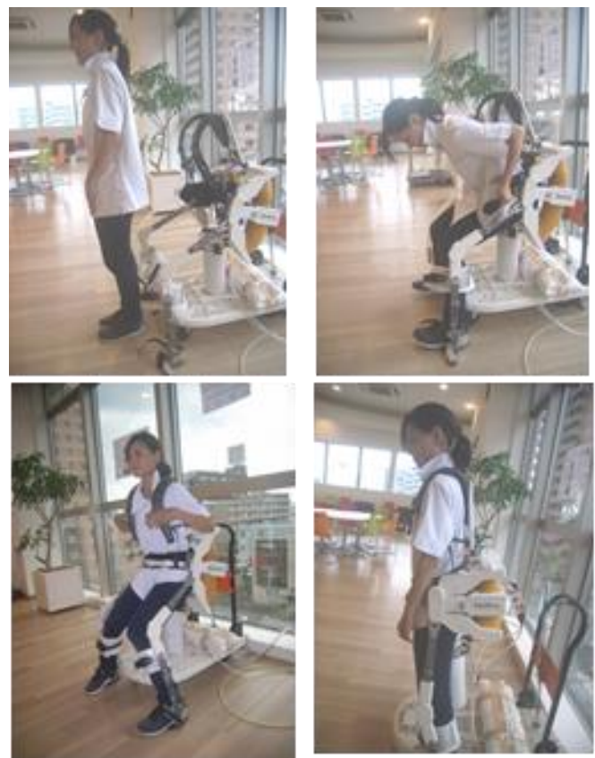
Fig.4 The desorption work of power assist suit can be done by herself
