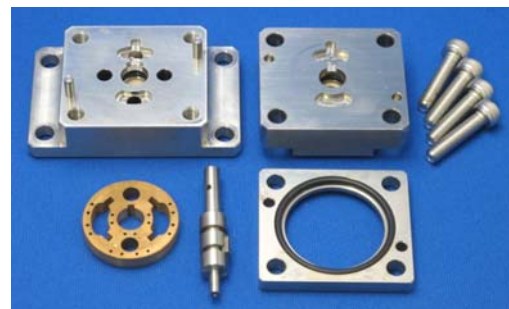
Fig. 2 Parts of the rotary-type four-way valve
