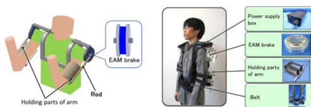
(a) Schematic diagram (b) The actually developed orthosis Fig.8 Upper limbs holding orthosis
