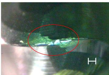
Fig.6 Observed flank wear in milling experiment
