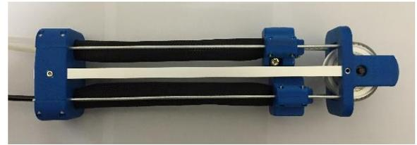
Fig.5 Prototype of Actuator
