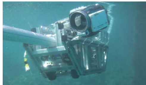
Fig.6 Gondola sliding along the fire hose inside the sea
