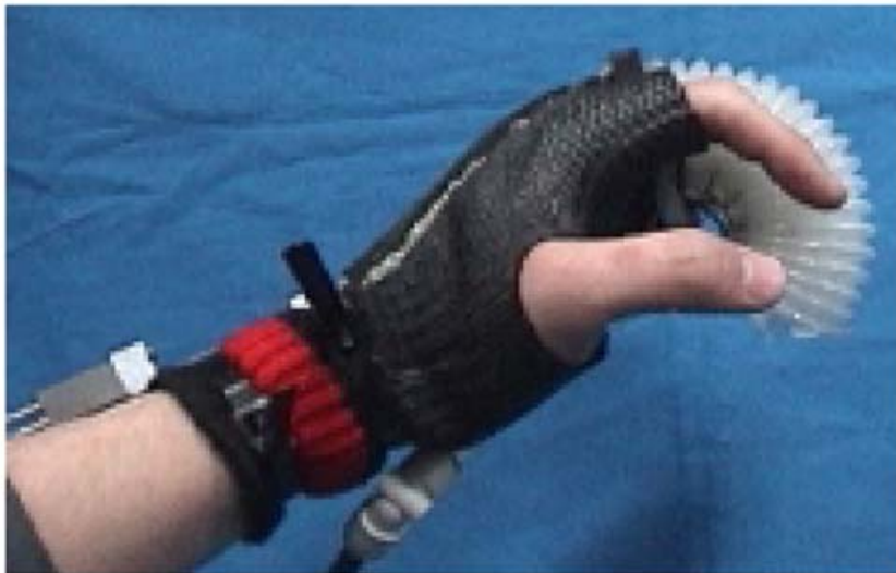
Developed WTA for a finger on right and the wearable valve on left.
