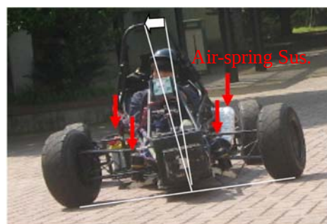
Fig. 5 Test vehicle in posture control (in anti-roll compensation while turning right)
