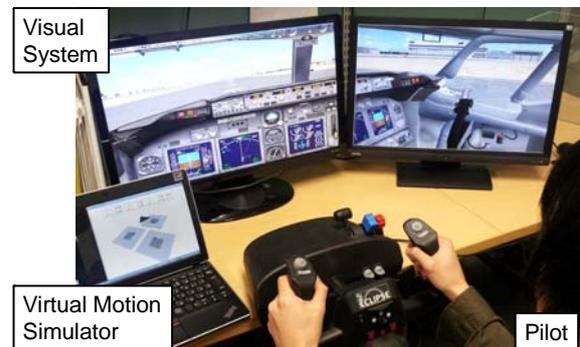
Fig. 5 Analysis of motion by pilot through visual system
